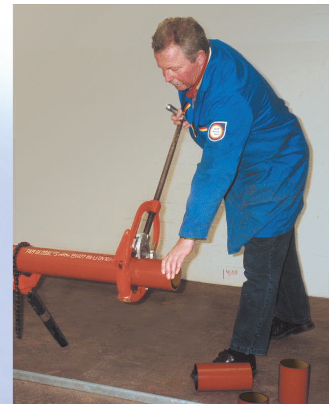
For easy cutting a simple hand-operated pipe-cutter suffices.
