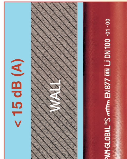
Cast iron with lamella graphite: high area weight, better airborne noise absorption.
